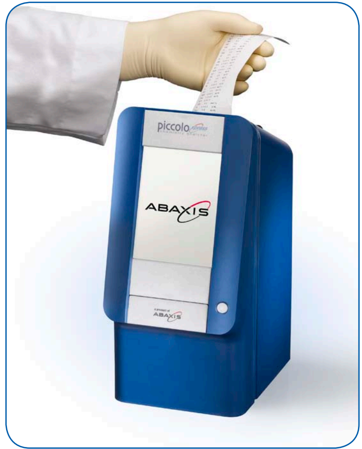
Step 3. After 12 minutes of processing time, the results are printed onto adhesive-backed thermal roll tape.
