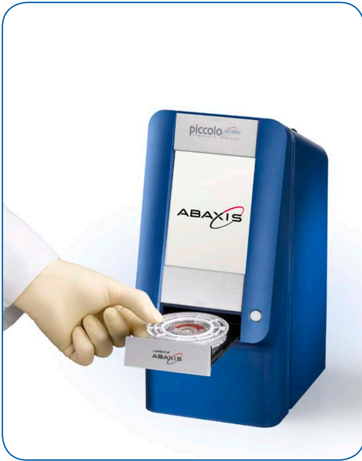
Step 2. Drawer is opened and full reagent disc is placed onto the receiving tray.
