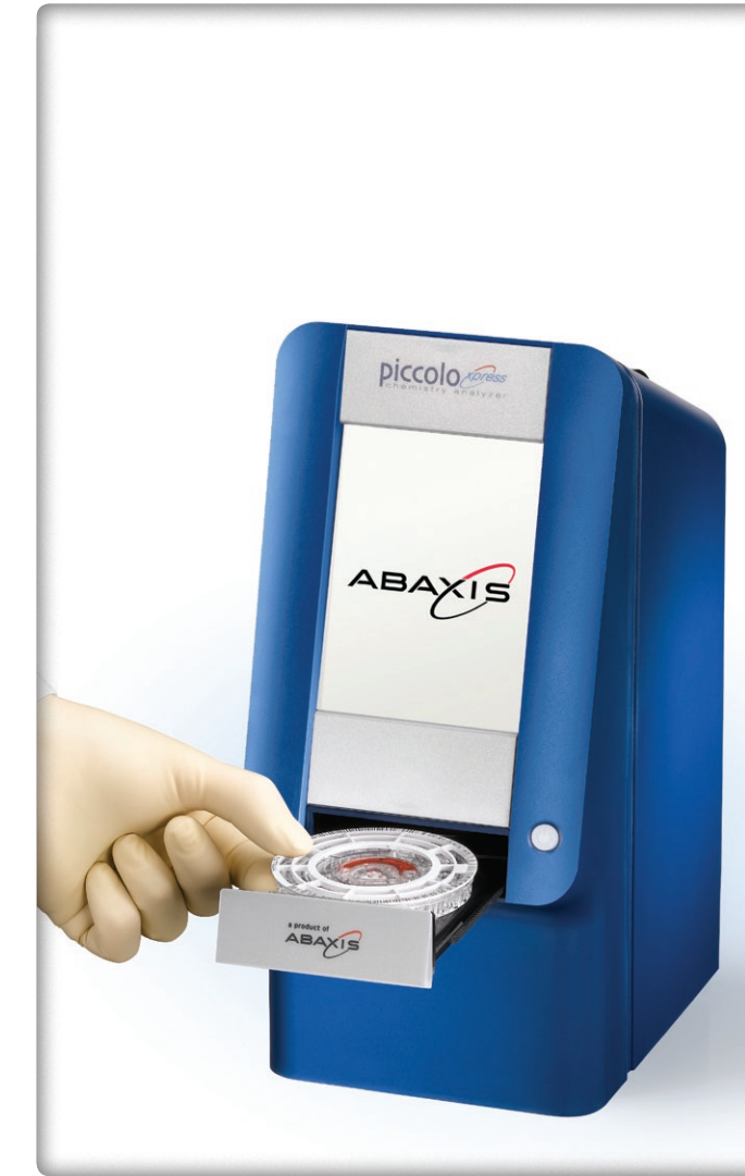
STEP 2. DRAWER IS OPENED AND FULL REAGENT DISC IS PLACED ONTO THE RECEIVING TRAY.
